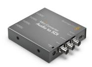
Embed audio into any SDI source in SD and HD formats up to 1080p60! Audio is input as balanced analog or AES/EBU using  $\frac{1}{4}$ " connectors from equipment such as mixers and analog decks. Mini Converter Audio to SDI is the ideal SD/HD SDI audio embedder for when you don't need the cost of the Ultra HD model!
