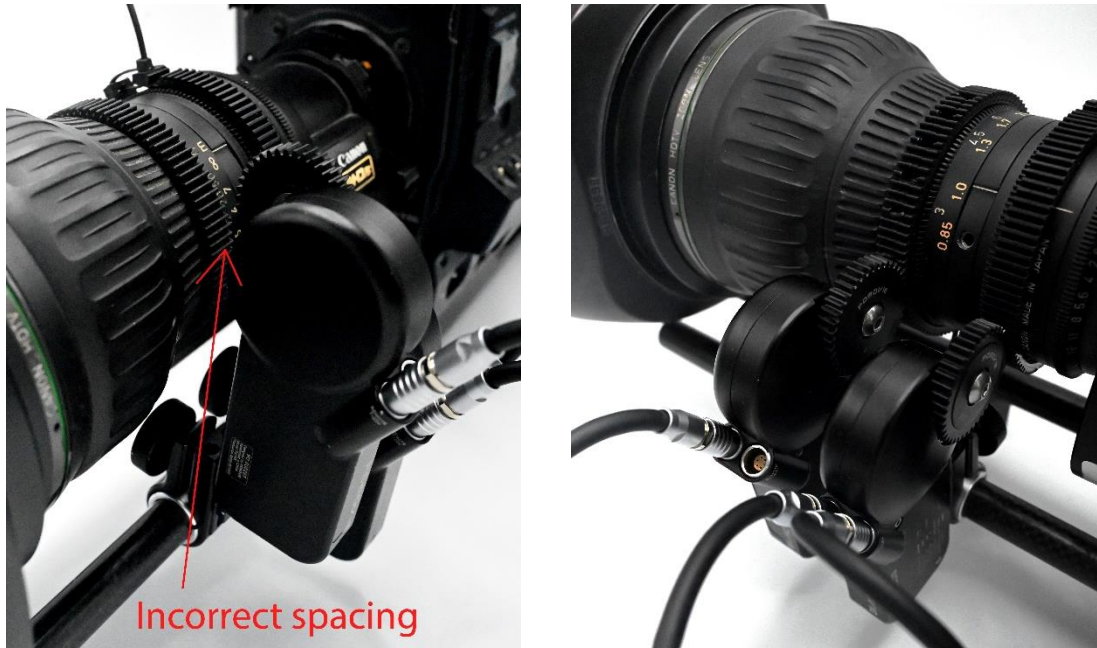
Figure 22: Incorrect and correct lens motor alignment
