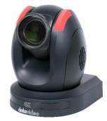
PTC-280 is our first UHD PTZ camera with full 50/59.94/60 output. Is has a 1/2.5" CMOS sensor for AV applications with a 12x optical and 16x digital zoom. There's a dual encoder built in, so next to HDMI and 3G-SDI output you can also stream in UHDp30 resolution. Optional NDI-HX module available!
